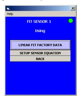
The user can activate the field calibration or the factory calibration. Selecting "Fit Data" menu allows the user to select which calibration the system uses to Display results. This is intended to give the user the ability to switch between Factory and Process Calibration as a method of checking the existing primary calibration or performing a new primary calibration.
