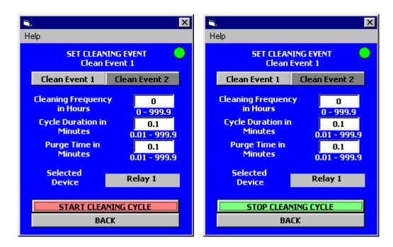
When manually starting a cleaning cycle make sure you have the variables set properly and a device selected.
