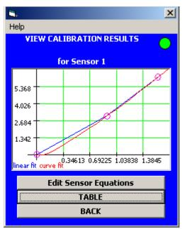
➤ Using "Fit Data" menu you may select either to use the Factory or Process calibration for sample analysis. You may select "Factory Calibration" data as reference but in most cases the process calibration will be more accurate as it represents the sample and not the factory standards.
