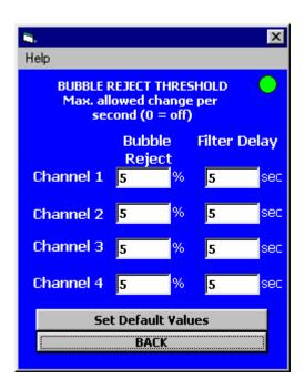
The Messenger also includes a feature that allows the customer to dampen the response of the system, by including added signal filtration. A unique bubble reject feature is also available; this feature allows the system to reject spurious signals caused by bubbles presence. The factory default is set for 5% and Filter
