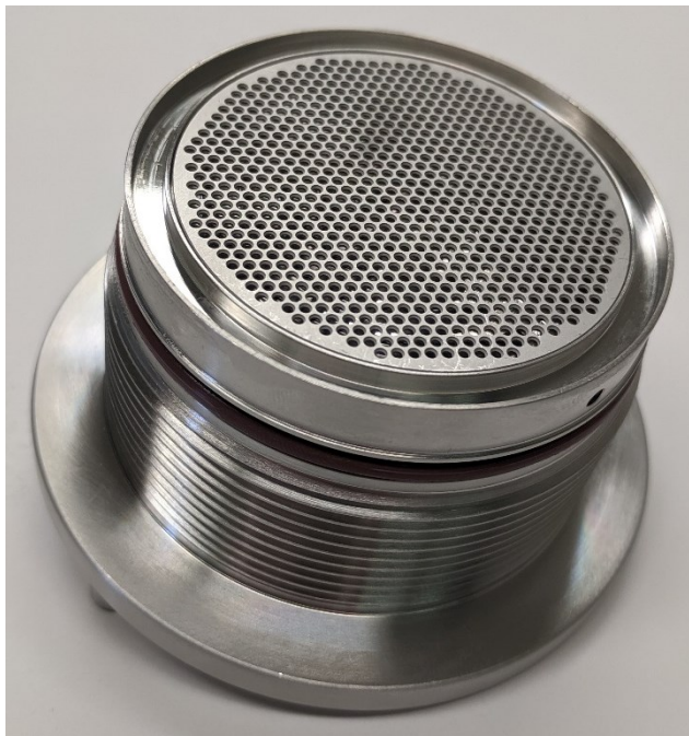
Figure 86: Liquid Membrane Separator Cover with Exposed Membrane Support
