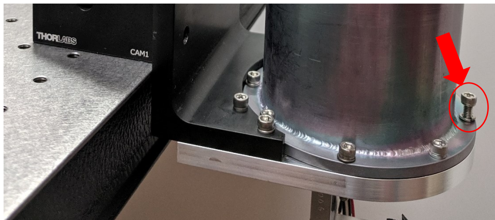
Figure 69: Screws Holding Herriott Cell Cover in Place
