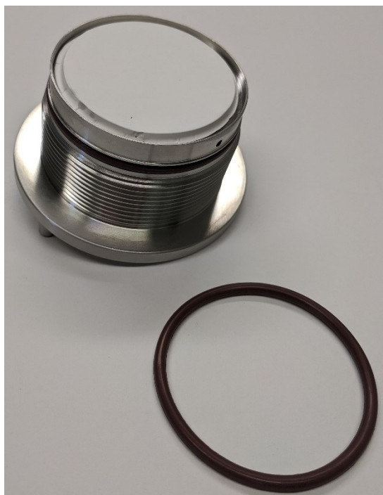
Figure 85: Liquid Membrane Separator Cover with O-ring Removed
