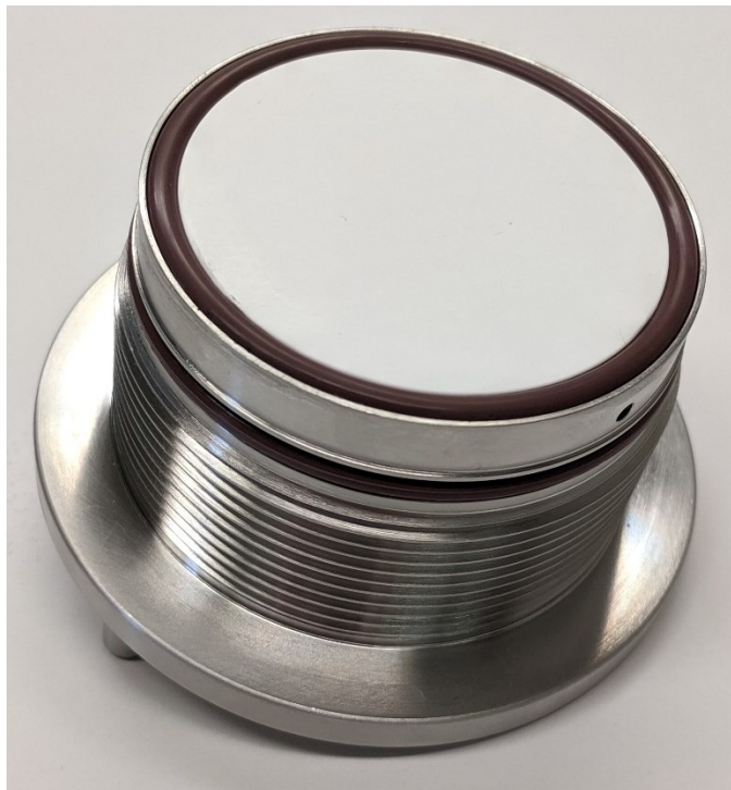
Figure 84: Removed Liquid Membrane Separator Cover
