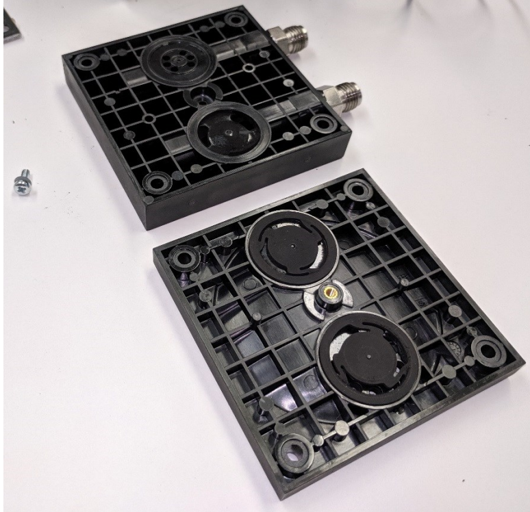
Figure 80: Separated Pump Head Plates
