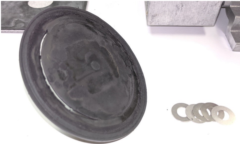
Figure 77: Torn Diaphragm and Diaphragm Spacers
