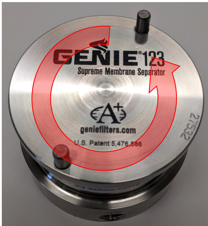
Figure 82: Unscrewing Liquid Membrane Separator Cover
